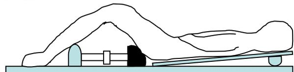
Fig. 3 Device utilized to compress the gluteus and simulate seating pressure inside the MRI magnet.
