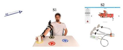
64472) is aimed at tuning and validating advanced, robot-based technologies supported by FES to facilitate recovery of arm and hand function in stroke survivors. RETRAINER includes two subsystems: S1 is a 3 degrees of freedom exoskeleton combined with FES provide triggered by **EMG** to additional support to the weakest
