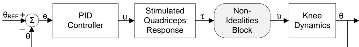
Fig. 1: Block diagram of simulation of PID control of electrically stimulated knee angle  $\theta$ .
