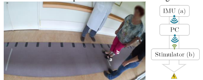
Figure 3 The subject is equipped with an inertial measurement unit (a) and a wirelessly programmable stimulator (b) connected through a PC.
