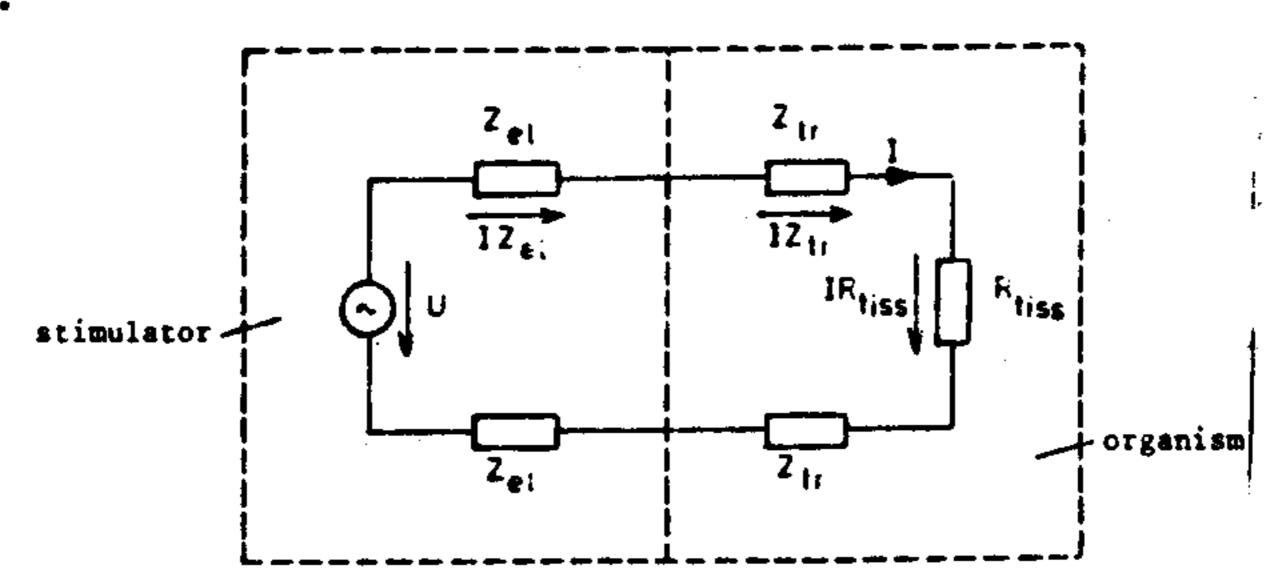
Fig. 1: Simplified electrical circuit diagram of a stimulator, the transition impedance, and the tissue to be stimulated under neglection of Z par.
