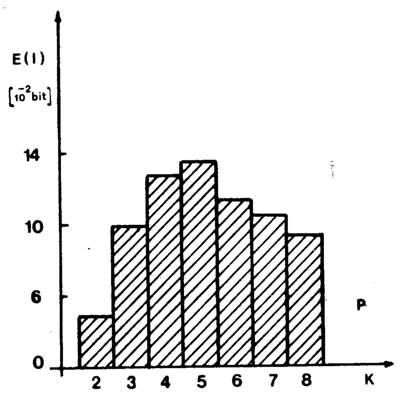
Fig.1 Histogram of the average mutual information content E(I) of parameters depending on K where K means the number of typical gait classes, K=1,2,...8
