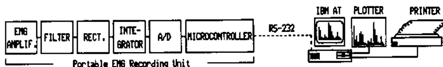
Fig. 1: Microcomputer based portable long-term sEMG recording system. Surface EMG signal is amplified, rectified, integrated, converted into digital form and stored into microcomputer memory. After 24 hours, accumulated data is transferred via serial link to the host computer. Data is there further processed and displayed in numerical and graphical form.
