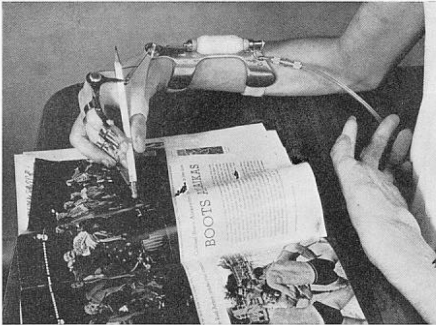
Figure 1. An externally powered finger prehension orthosis with wrist friction joint is used to restore function for the patient with a spinal cord lesion at the C-5, 6 level
