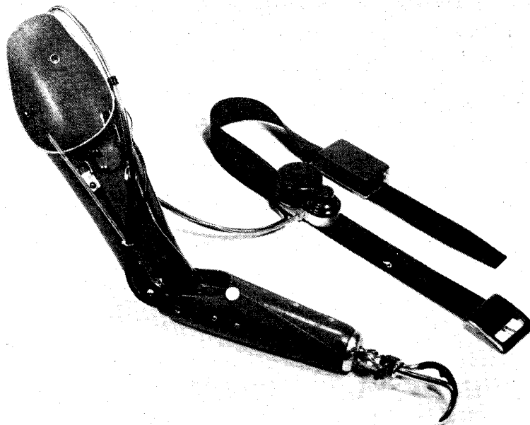
Fig. 8. HT - elbow disarticulation prosthesis. Belt mounted battery and motor. Myoelectric sensor in socket wall. Outside locking elbow hinges.
