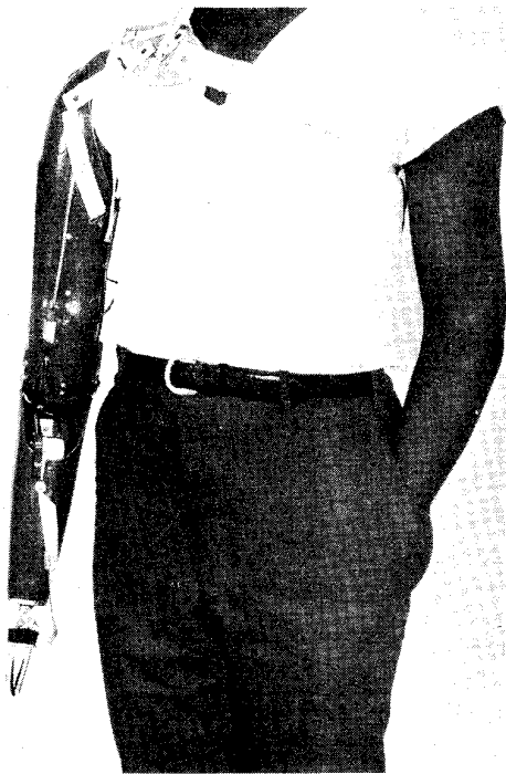
Fig. 10. LB - above elbow prosthesis motor in elbow. Battery clips to belt. Myoelectric sensor in socket wall over biceps.
