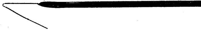
Figure 1. The Karma wire electrode in a hypodermic needle. 2.5 mm of the hook-shaped tip is deinsulated.
