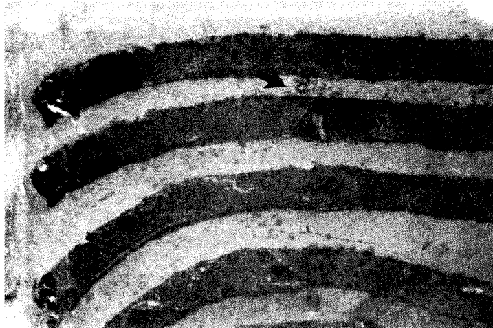
Figure 6: View onto the basic print of the implant (magn. 20X) with cavities and copper migration because of humidity and DC-currents which shunts the output
