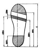
Fig.2. Contact transducers placement on the foot plantor surface
