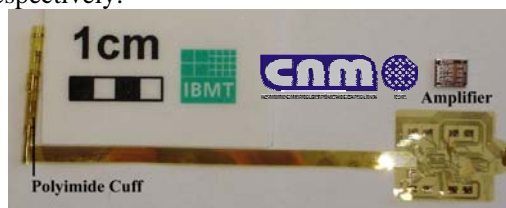
Fig. 1: Polyimide cuff substrate (1.6 mm dia.) after metallization of electrodes and conductive lines with amplifier before assembling.
