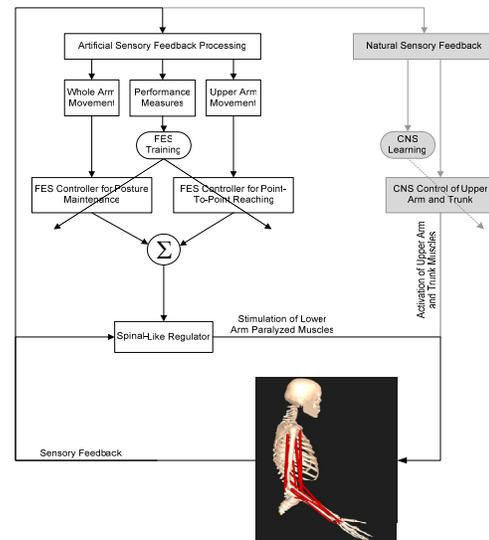
**Figure 2.** Biomimetic design for FES control of partially paralyzed arm. Upper arm movement is under voluntary control and could be modified by the learning process of the CNS. The movement of the paralyzed lower arm is controlled by the FES that takes advantage of circuitry and residual control in the CNS.
