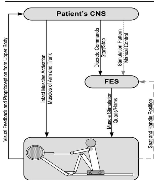
**Figure 1.** Two control strategies for man-machine coordination in FES rowing. In manual control (dotted line), the stimulation of paralyzed muscles is controlled by a continuous command from CNS. In automatic control (dashed line), prosthetic sensory feedback are used by FES controller to determine the timing and pattern of stimulation.
