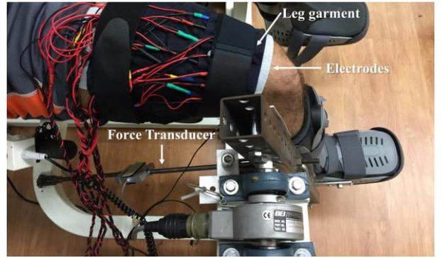
Figure 1. Participant seated in the LEM while wearing the garment, which contains the vibration motors. The pair of electrodes reside below the garment in the proximal and distal part of the quadriceps muscle group.
